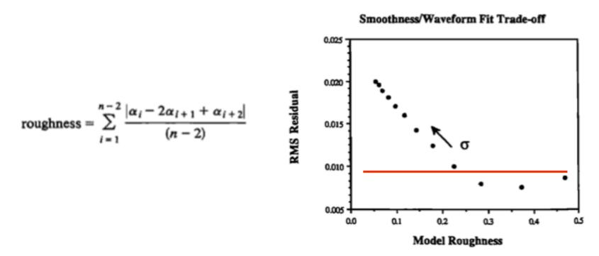
A value for  $\sigma$  is chose, for instance, from the noise level from the transverse RF.
